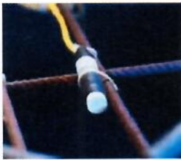
Fig 13. Embedded reference electrode for CP [7]
